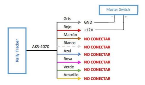
The device supplied by Al Kamel Systems must be powered from the vehicle battery. The voltage must be between 9V and 15V. It is strictly forbidden to install any switch or circuit breaker between the equipment and the battery, the power supply must be direct and only interrupted by the Master Switch of the vehicle.
